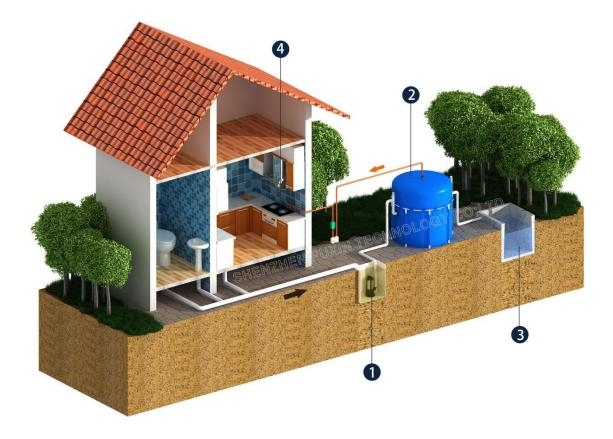
1.feeding pump, 2.digester, 3.slurry pool, 4.biogas stove
