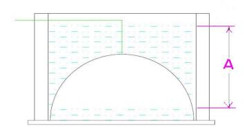
The pressure is caused by the distance between water level of gasholder and water level of concrete tank
