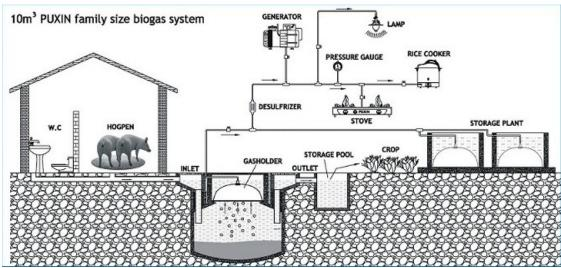
With 10 m3 family size Puxin biogas plant as per the above drawing, enough biogas can be provided to 2 families of 4 persons each for cooking and lighting. The digester is made of concrete.
